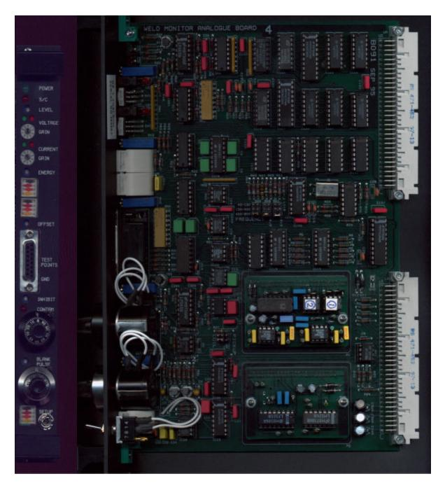
The Vertex Mk.IV Analogue Board for the WM-3 series of weld monitors is a plug-in replacement for earlier versions of the Analogue Board. It offers improved performance and maintainability. With its optional current pickup it can be used on lines equipped with the new 'Unisoud' power supply. This is the only way the Monitor can continue to be used when the Unisoud power supply is fitted.
